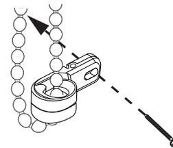
Then secure to the mounting surface using the screw provided
