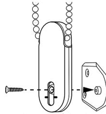
Insert the nub of the Bracket into the Cord Tension Lock and secure with small screw provided
