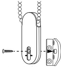
Insert the nub of the Bracket into the Cord Tension Lock and secure with small screw provided
