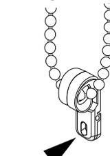
With the shade securely installed, pull the chain taut and mark the location on the mounting surface
