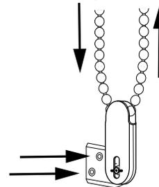
While holding the lock firmly in place, check if the loop can move freely through it and then mark holes
