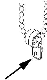
With the shade securely installed, pull the chain taut and mark the location on the mounting surface
