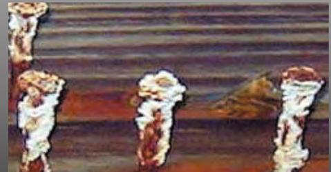
Name Brand hot dip galvanized fastener after 1008 hours salt spray
