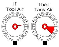
Compressor tank air must be maintained above the pressure supplied to the tool
