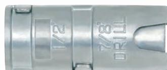
Aerosmith®'s Machine Bolt Anchors can be used in concrete, block, brick and stone. The anchor consists of a set of expansion shields and an expander cone. The product is manufactured from zinc alloy. As the anchor is tightened, the cone gets drawn into the expansion shield which compresses them against the base material. This product is not recommended in overhead applications.
