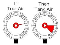
Compressor tank air must be maintained above the pressure supplied to the tool
