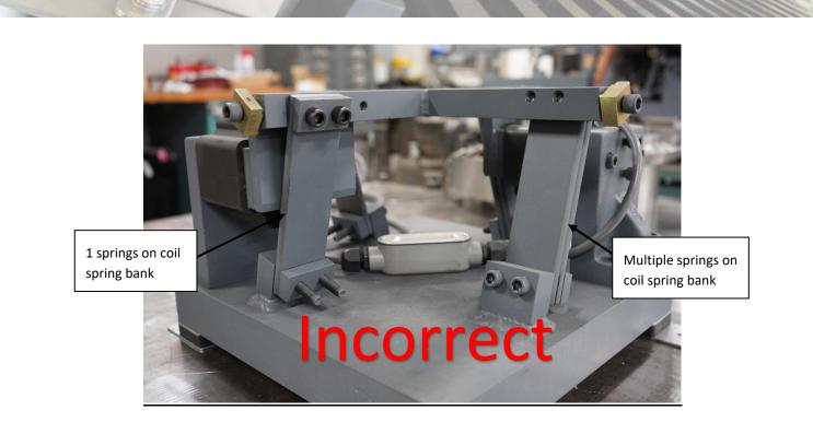
c. When multiple thicknesses of springs are required to achieve proper tuning, always install thicker springs closer to the cross arms (example shown below).
