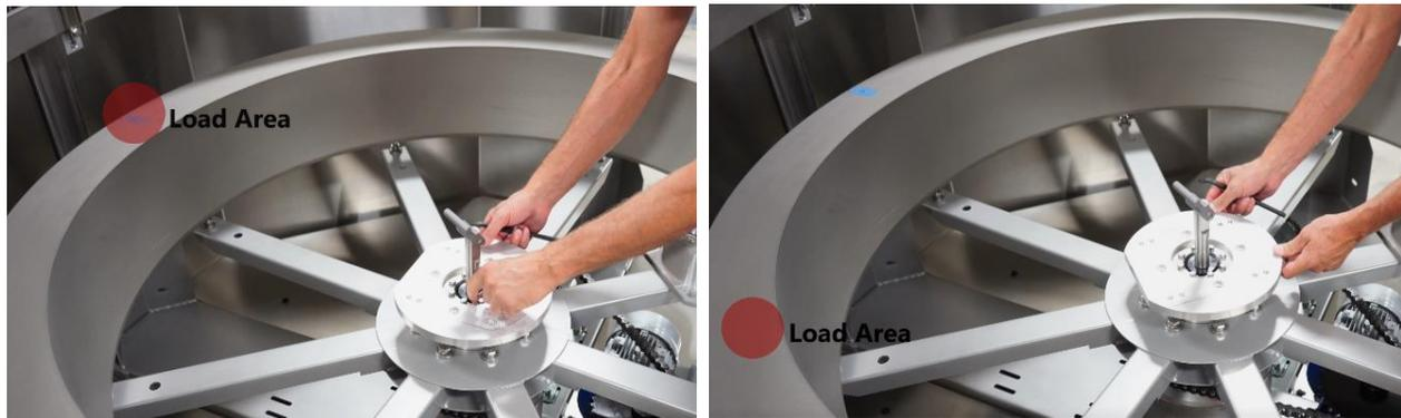
11. Reinstall the (4) 12 mm socket-head bolts using the pre-drilled holes below to firmly secure the Mounting Plate in the new desired location.
