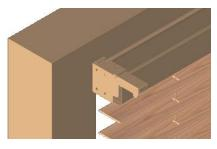
Close the lid of the bracket, making sure that it snaps in the down position.
