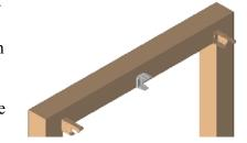
• Install two screws to attach the bracket.
