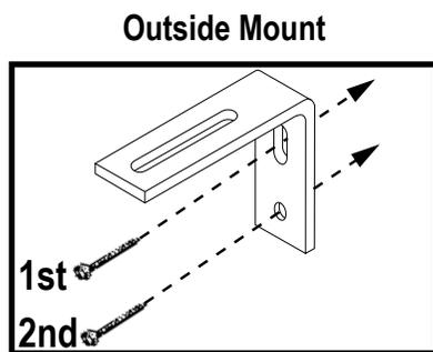
Begin installing the brackets by using the elongated hole first in case any adjustments must be made.
