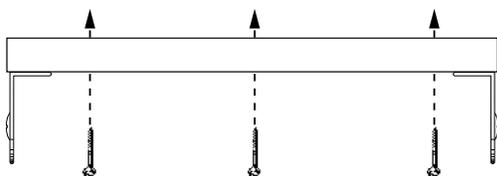
Space screws the same way brackets would be spaced. 3 1/4" in from the ends and evenly space the rest needed given your opening width and mark where holes are needed
