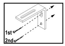
Begin installing the brackets by using the elongated hole first in case any adjustments must be made.
