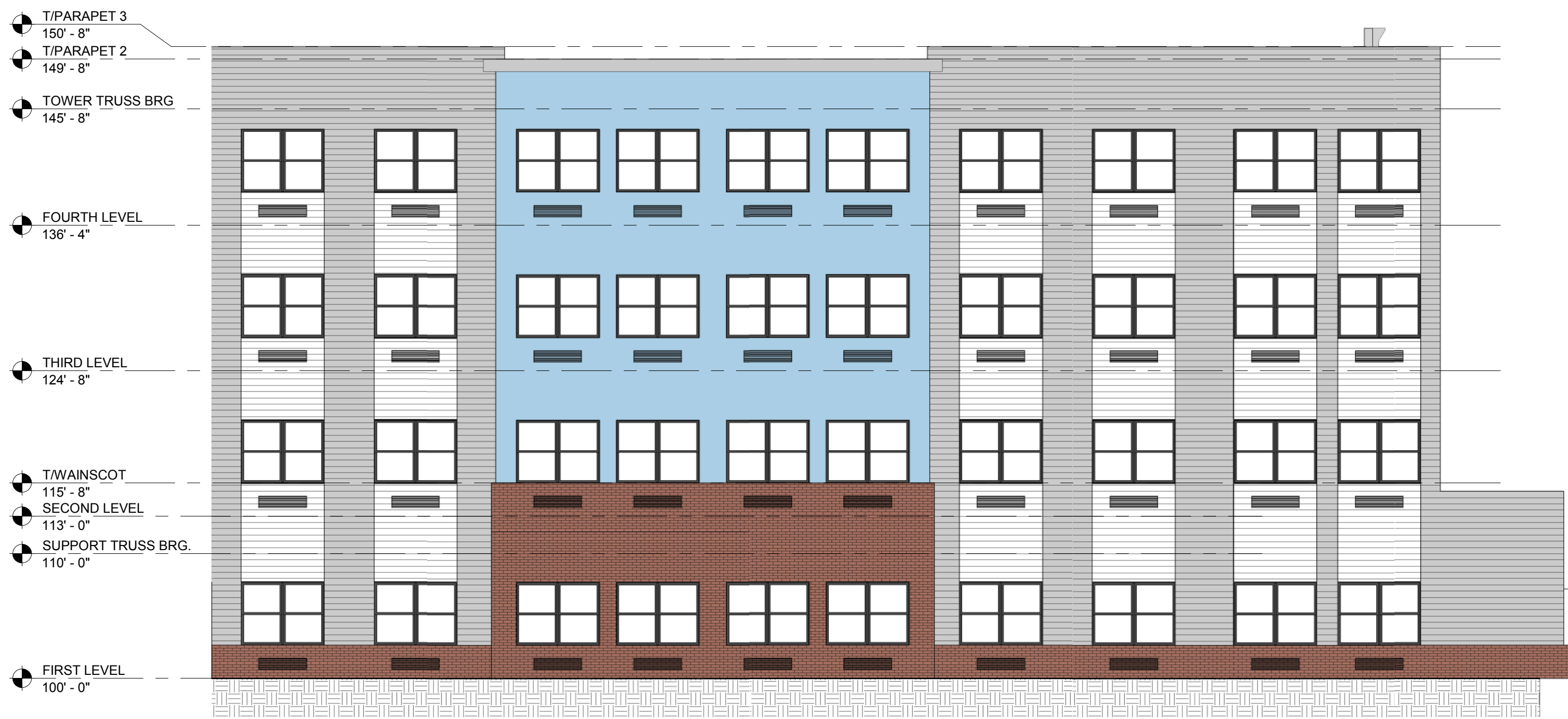
4 SOUTH WING ELEVATION 1/8" = 1'-0"
