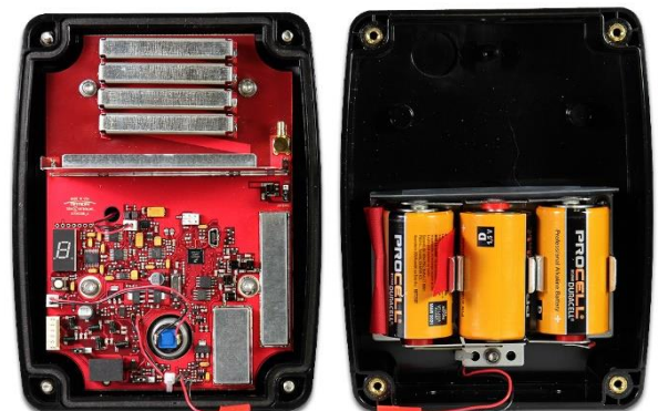
Q-Series power cable disconnected during battery installation
