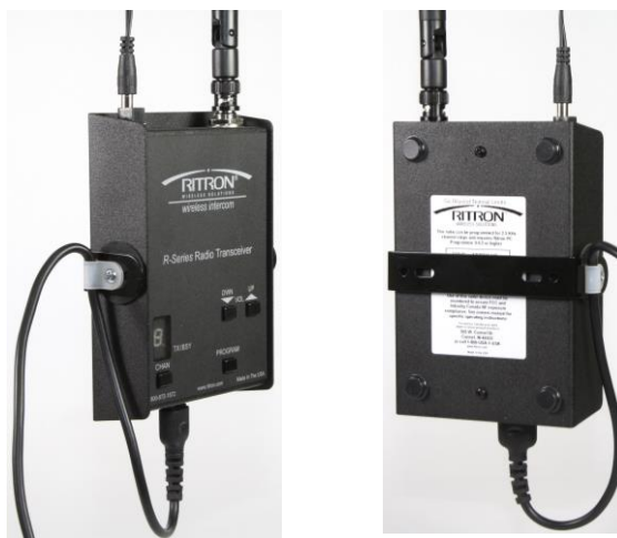
Figure-3: R-Series Radio Installation
