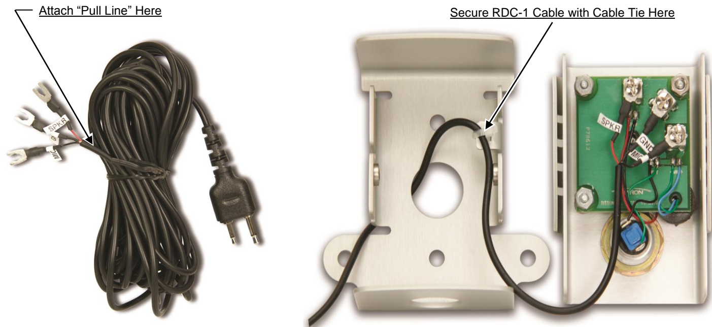
Figure-2: RDC-1 Installation
