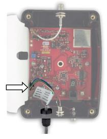
7. Pull cable assembly 60201127 through the strain relief from the inside as shown. Plug the cable assembly into the pcb connector and tighten the sealing nut.
