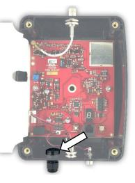
Install the Heyco strain relief included with cable assembly 60201127. Do not tighten the sealing nut at this time.
