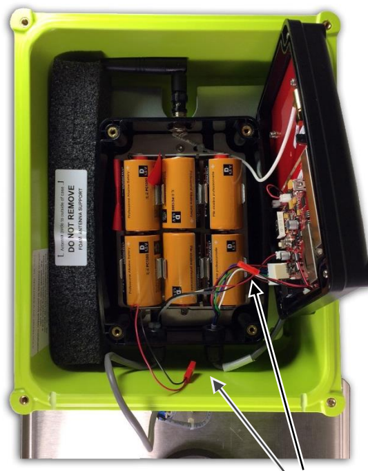
XT-Series battery cable disconnected during battery installation
