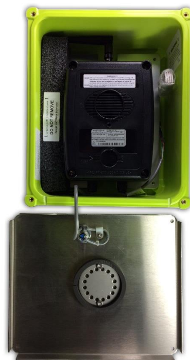
XT-Series case with metal faceplate removed
