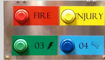
*Call stations are located throughout the operation and include color-coded buttons that activate custom two-way radio alert messages for fire, injury, electrician needed, and millwright needed.*
