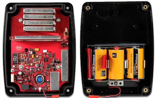
Q-Series power cable disconnected during battery installation
