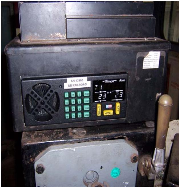
Ritron's clean cab radio, designed specifically for the railroad industry, is a dual mode radio with an easy upgrade path to digital operation. Railroads are taking advantage of this economical option since it can be quickly upgraded to tri-mode with the addition of a circuit board and a software upgrade.
