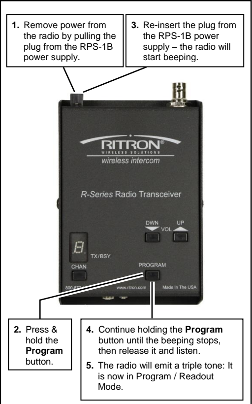
Figure-2: HOW TO PLACE THE RADIO IN PROGRAM / READOUT MODE
