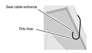
FIG-7: Outside Antenna Cable Installation
